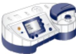
Choose the cell-type specific program. Insert the cuvette into the Nucleofector and press the "X" button to start the program.
